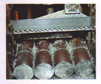
Cutting is the first step in the manufacturing process of any fastener. Raw material in the form of round or Hex bar is either saw cut or sheared to the desired length. Bandsaws use saw blades to cut through the steel round bar. On the other hand, shearing equipment functions like a guillotine, "chopping" the raw material. During the shearing operation, the material is automatically run against a stop and then sheared to length.
