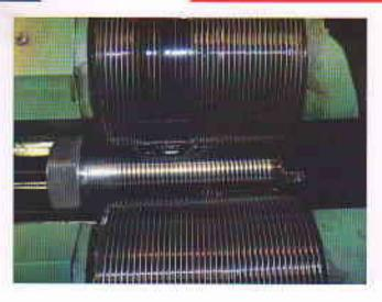
Thread Rolling is a metal rolling process used extensively in manufacturing of screws, bolts and other fasteners. Thread rolling involves forming the threads into the metal of a blank by a pressing and rolling action between two die. The die surfaces hold the shape and the force of the action forms the threads into the material.
